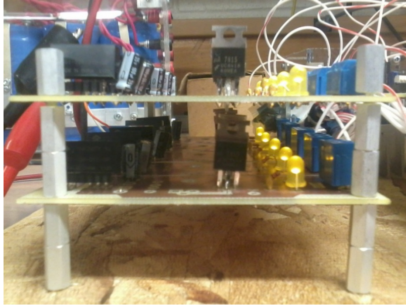
Figure F.7 Laboratory prototype of isolated power circuit.
