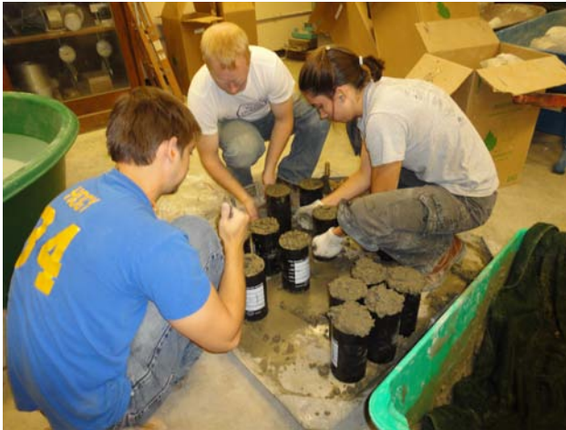
From left: Undergraduate assistant Josh Hogancamp, CESR MS student Aaron Crowley, CESR MS student Samantha Jeffries are making higher volume fly ash concrete for testing as part of the MS research of Crowley and Jeffries.
