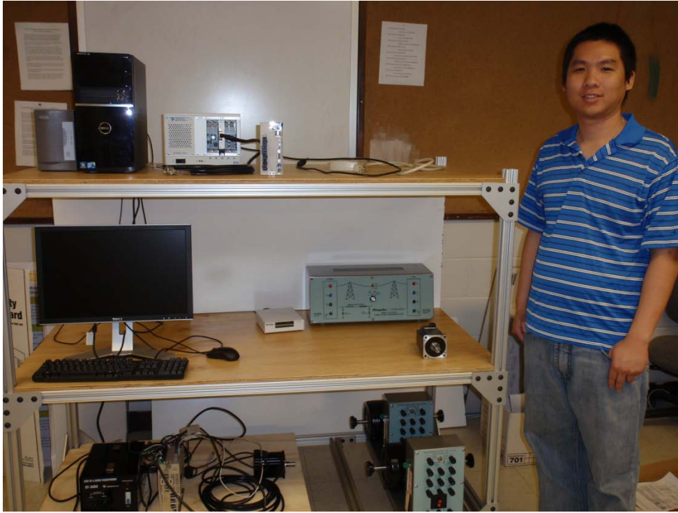
Figure 2 Labgrid pictured with two generators a transmission line and data acquisition system.
